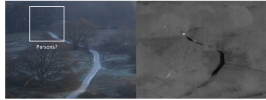
Figure 2 Loss of visibility of humans in the shades of the trees with VIS (left) but clear visibility with LWIR (right).
