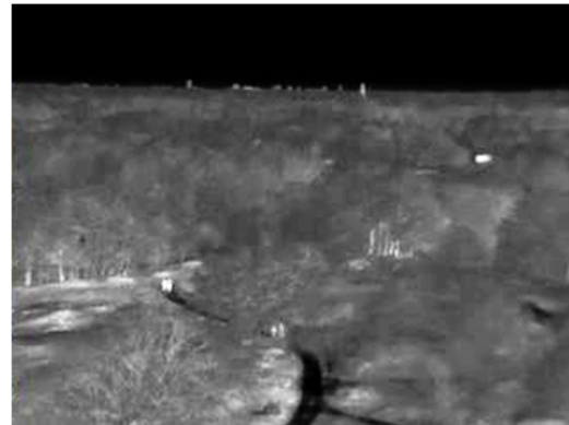
Figure 6 LWIR view of the scene. One can recognize people (blobs) walking on the cold path (black track).
