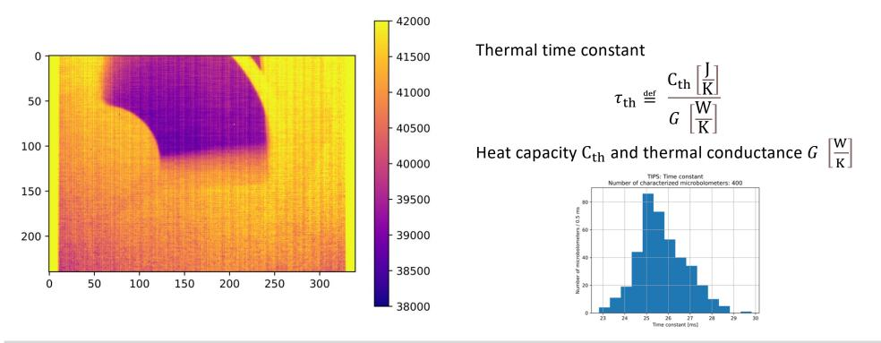
Preliminary: Thermal time constant of about 26ms (for these microbolometers)
