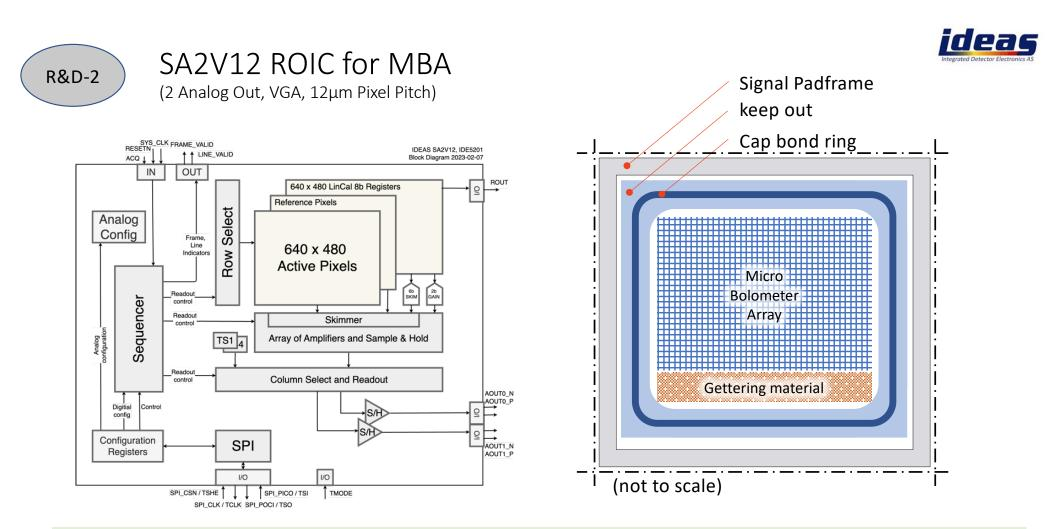
Block diagram of the ROIC, to be manufactured in CMOS. The Microbolometer array will be fabricated directly on the ROIC.
