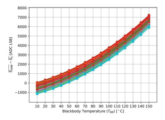
SITF – signal transfer function  $\overline{S}(i, j, T) \text{ [LSB]} \stackrel{\text{def}}{=} \frac{1}{200} \sum_{k=1}^{200} S_k(i, j, T) \text{ [LSB]}$ Responsivity  $R(i, j, T) \left[\frac{\text{LSB}}{\text{K}}\right] \stackrel{\text{def}}{=} \frac{\partial P(i, j, T) \text{ [LSB]}}{\partial T \text{ [K]}}$ With P(i, j, T) is polynomial fit to  $\overline{S}(i, j, T)$ .
