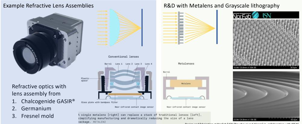
Design and fabrication at NorFab/USN [Bouchouri and Akram] in collaboration with IDEAS. Lens of f/2, Ø8mm, 10µm CWL monochrome, silicon pillars of 6.3µm height and 5µm pitch.
