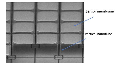
SEM-picture of the nanotube-microbolometers
