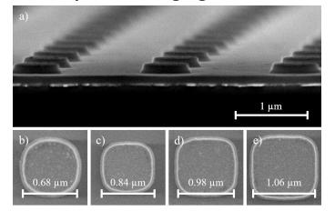
SEM-picture of fabricated MIM test structures
